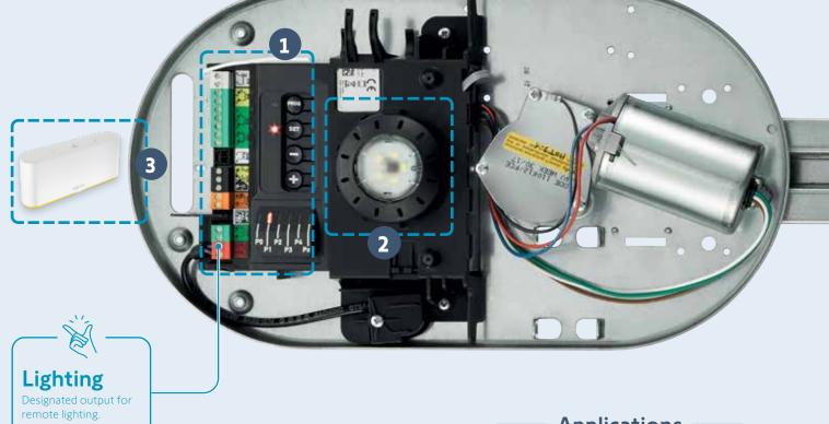
remote lighting. Automatically switched on with the garage door, and coperated separately.
